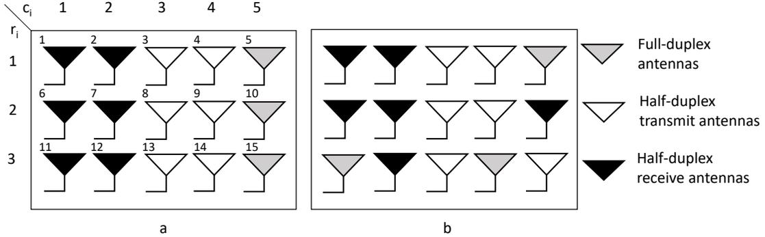
Fig. 1: Two example configurations for an array with  $M = 15$ , with  $N_{ac} = 3$  analog cancelers. For each configuration,  $M_r = M_t = 9$ .
