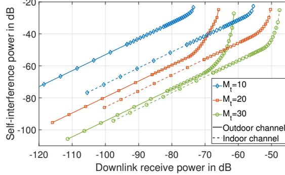
(b) *Self-interference suppression and downlink receive power of JointNull for the configurations with  $M_t = \{10, 20, 30\}$  in outdoor channel conditions.*
