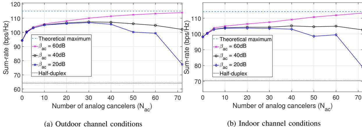
Fig. 6: The  $N_{ac}$  that achieves maximal sum-rate with JointNull depends on both the quality of analog cancelers and the channel conditions.
