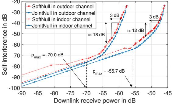
(a) *JointNull and SoftNull comparison for a configuration with  $M_t = M_r = 36$ . The self-interference reduction and downlink receive power reduction are equal for JointNull when  $p_{dl} \leq p_{max}$  i.e., tradeoff curves are linear with unit slope for  $p_{dl} \leq p_{max}$ .*
