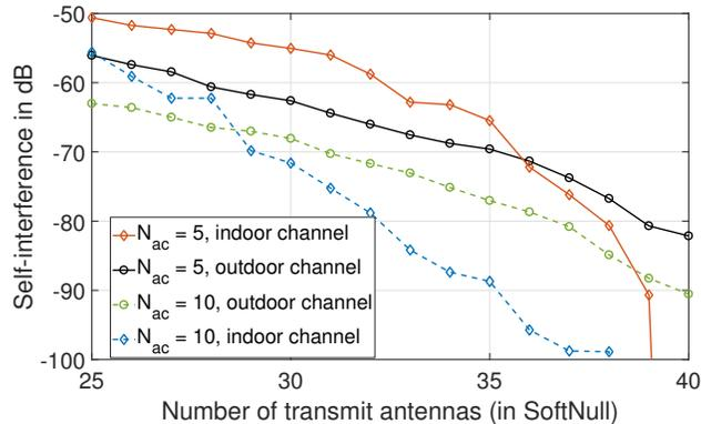
Fig. 5: For the analog cancelers,  $\beta_{ac} = 40$  dB. Self-interference for indoor channel decreases faster than outdoor channel after cross-over point.
