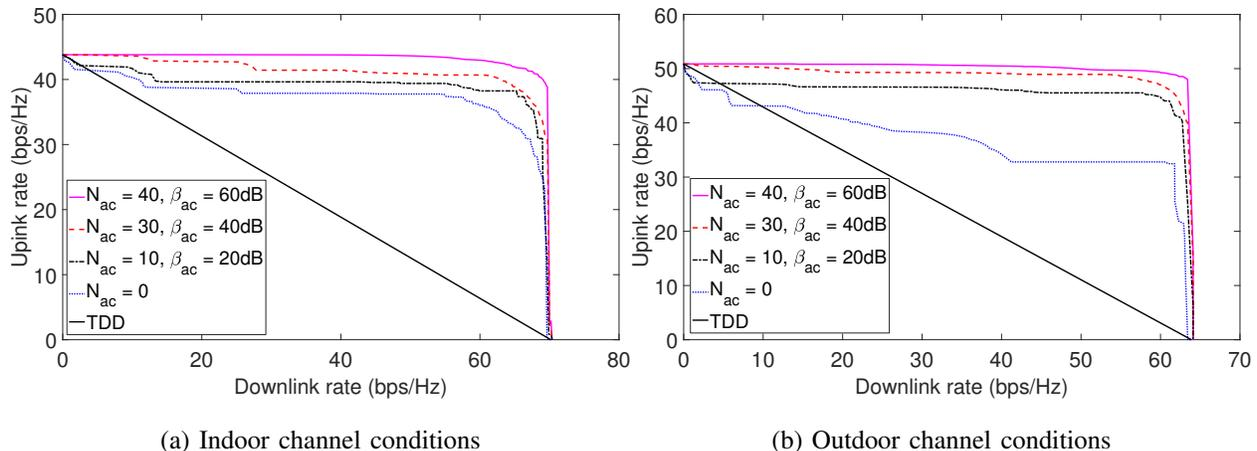
Fig. 7: Comparing JointNull achievable rates with TDD
