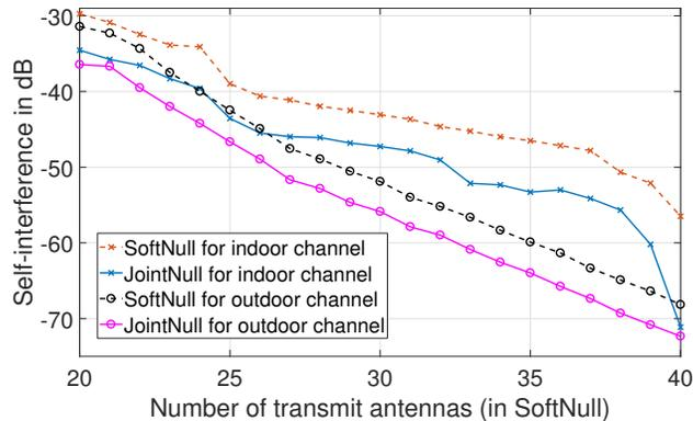
Fig. 4: Downlink receive power is fixed. The  $x$  coordinate is the number of transmit antennas for the SoftNull. The curves labeled 'JointNull' give the self-interference achieved by JointNull with the downlink and uplink receive power same as that of the corresponding SoftNull precoder.
